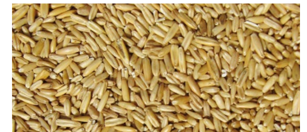
↑ Mixture of hulled and unhulled kernels as well as hulls downstream of the impact huller
