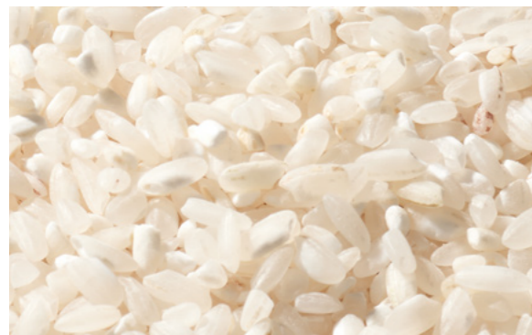
↑ Input product: coarse broken rice downstream of the plansifter for the indented cylinder
